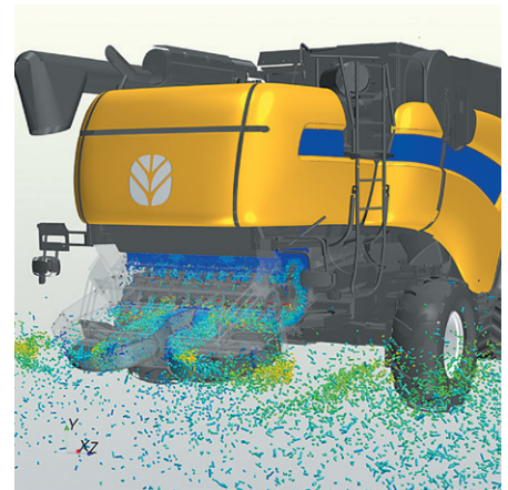
Combine harvester DEM simulation. (Courtesy: CNH Belgium N.V.)
